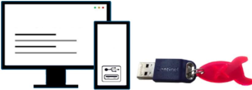
5. The Sentinel LDK communicates via TCP and UDP on socket/port 1947. This socket is IANA-registered exclusively for this purpose. It is therefore required that the firewall settings do not block the **port 1947**.
